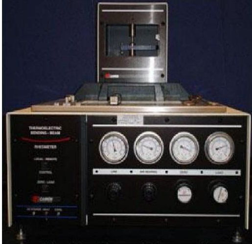
Figure 2.10: Bending Beam Rheometer (BBR) [51].
