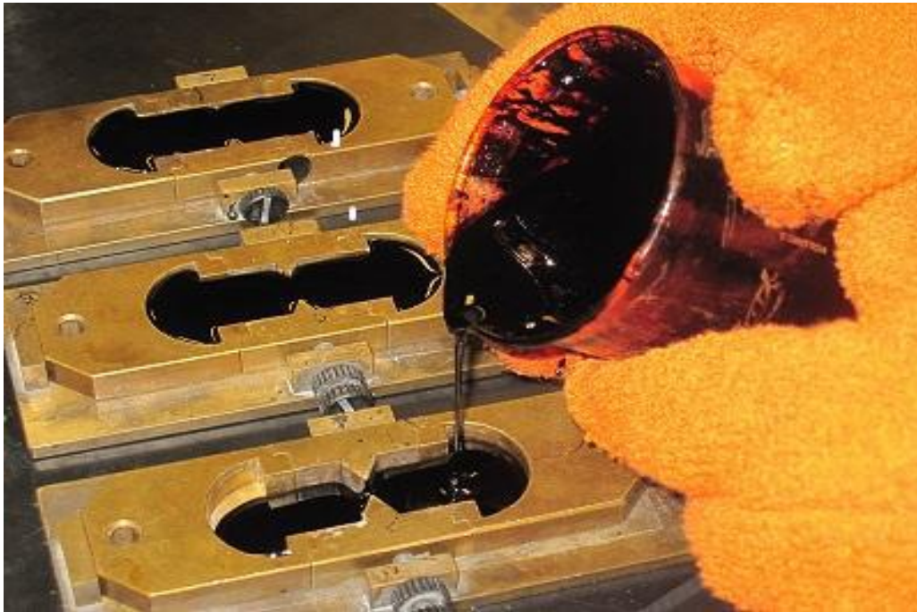
Figure 3.5 DENT sample preparation [11].
