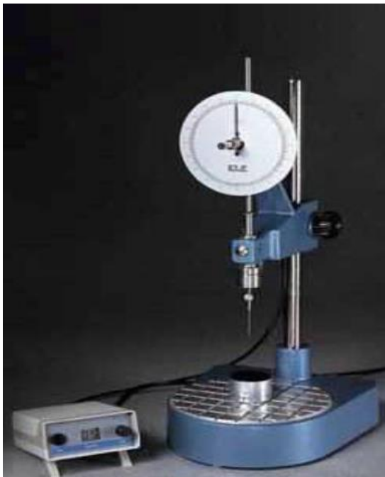
Figure 2.4: Equipment for testing penetration of asphalt binders [39].
