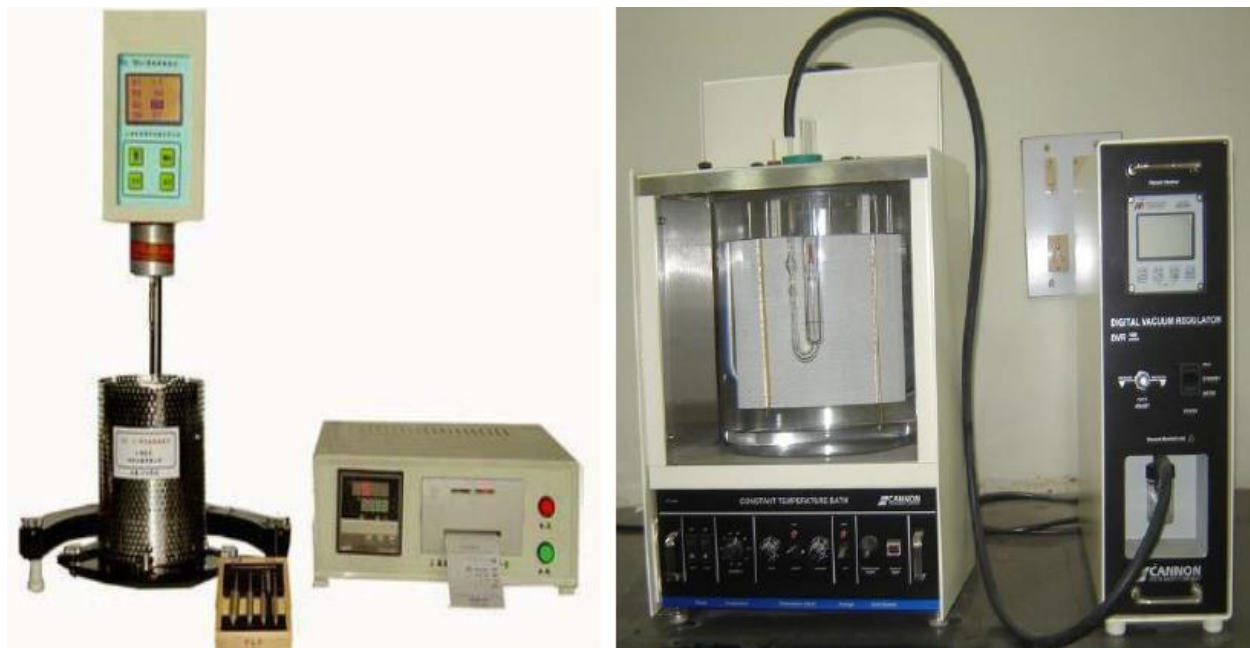
Figure 2.6: Brookfield viscometer and capillary viscometer [43, 44].
