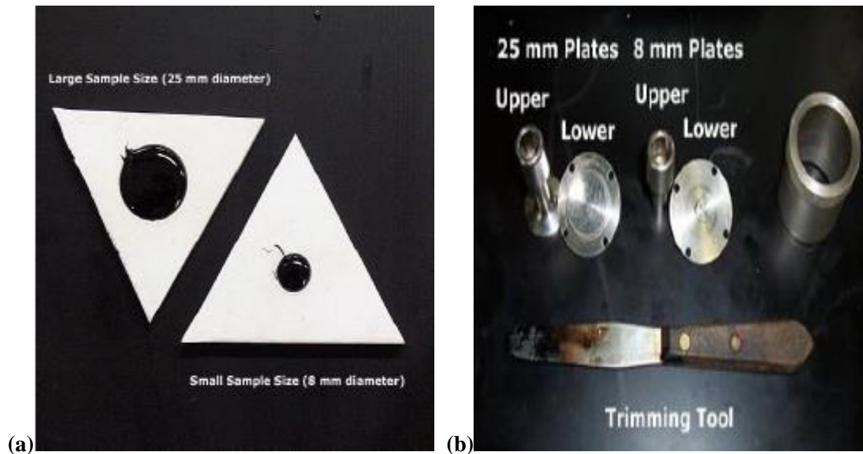
Figure 3.3 (A) DSR sample molds and (B) DSR test equipment [66].
