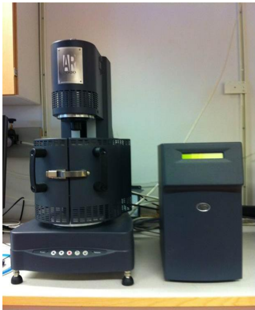
Figure 2.9: Dynamic Shear Rheometer (DSR) [47].
