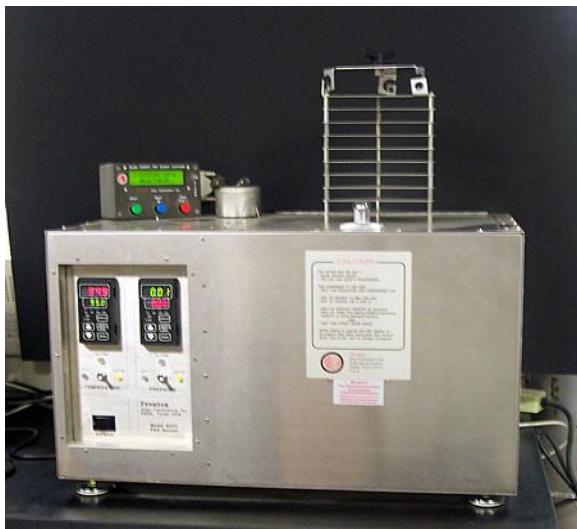
Figure 2.8: Pressure aging vessel [41].
