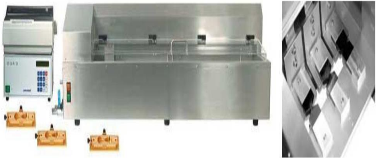
Figure 2.12: DENT test setup [6].
