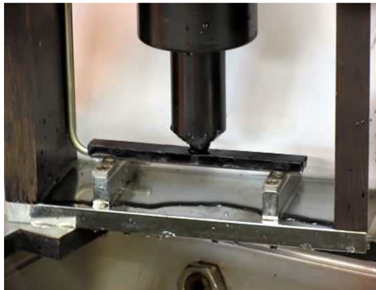
Figure 8: BBR beam on its supports [26]
