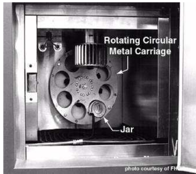
Figure 6. Rolling thin-film oven test [26].
