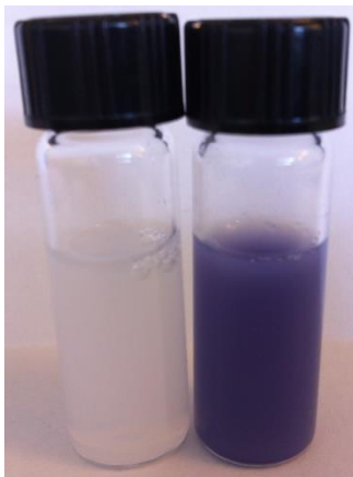
Figure 3-4 Photograph of vials containing small PS-NH 2 particles that were dispersed into distilled water (left) and into an aqueous ninhydrin solution (right).
