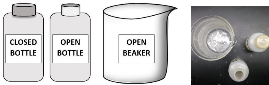
Figure 4.7: Schematic of closed and open 60-mL plastic bottles and a 40-mL glass beaker for exposure analysis (left). At right, a bird's-eye view showing potassium carbonate precipitate forming in the exposed fuel.
