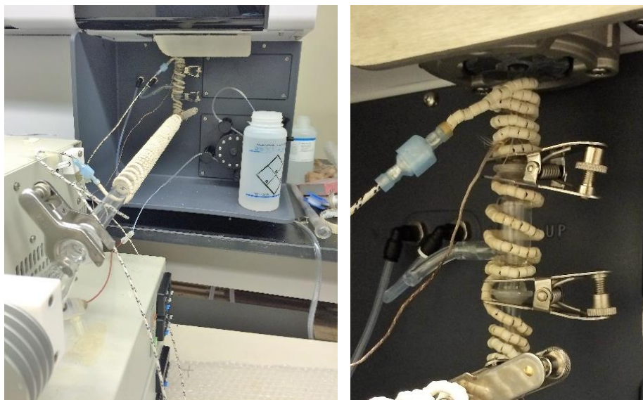
Figure 2.3: USN-PET(IR) setup for Agilent 5100; at left using a long pre-evaporation tube and L-connector (54 cm total); at right, the sheath adaptor and bottom 3 cm of the torch are heated, with thermocouple attached to the lower region of the torch injector.
