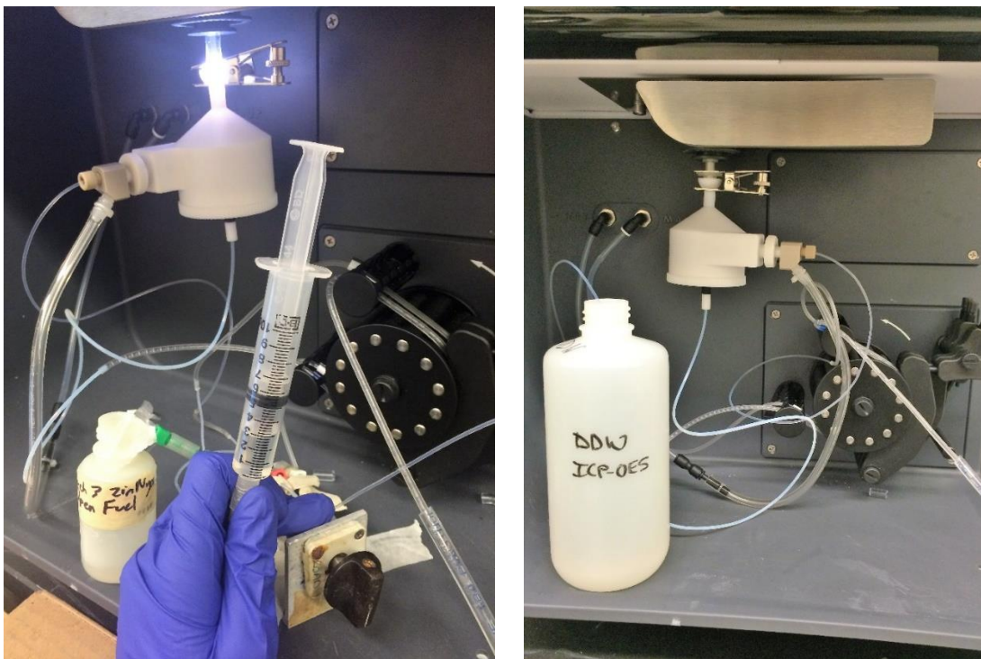
Figure 4.1: Sample introduction system consisting of a prototype V-groove nebuliser and an inert Teflon spray chamber; at left with a flow-injection switching valve, and at right without FI for dilution methods.
