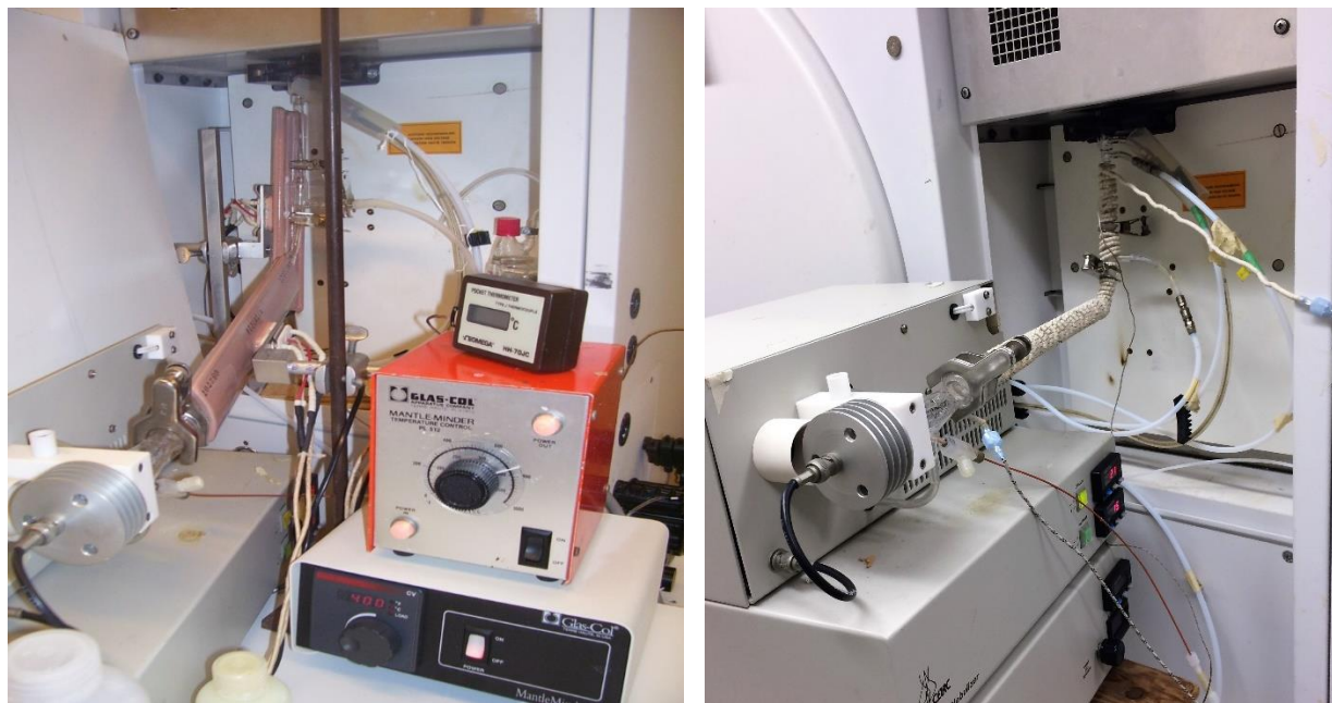
Figure 2.2: USN-PET(IR) setup for SPECTRO ARCOS ICP-OES with block infrared heaters (a) at left, and with a rope infrared heater (b) at right.
