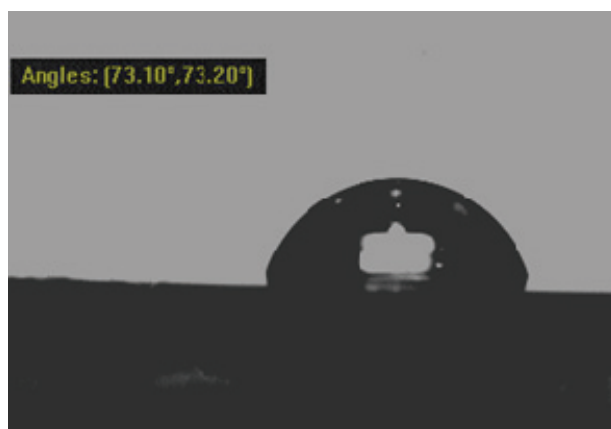
Figure 3-14 Contact angle measured for a water droplet on a PAEMA film substrate.
