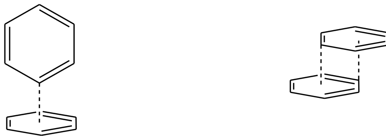
Figure 1.5 An edge-to-face interaction between the \sigma -scaffold of one ring and the \pi -cloud of the other ring (left). An offset face-to-face interaction between the outer \sigma -scaffold and center of both aromatic ring systems (right). 3,4,5
