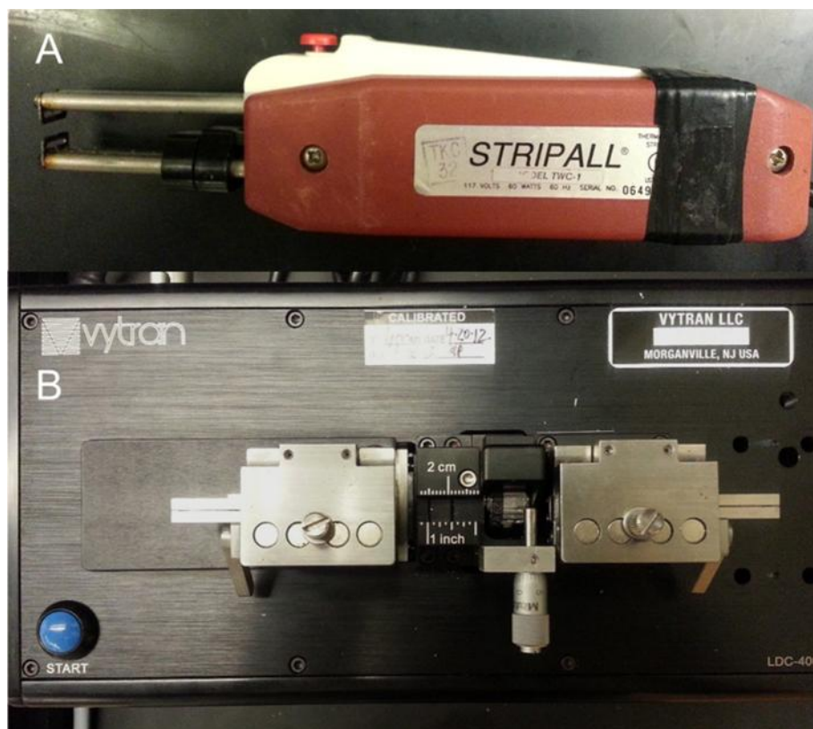
Figure 3.1 Pictures of A) the fiber coating remover: Stripall® and B) the precise fiber cleaver: Vytran LDC-400.
