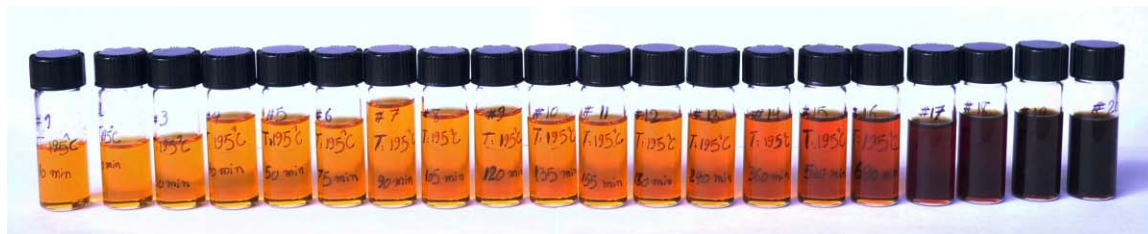
Figure 3.4 Photo of samples taken at different times when oil was heated to 195 °C. From left: fresh turbine oil, and samples taken at the same intervals as described in Figure 3.6.
