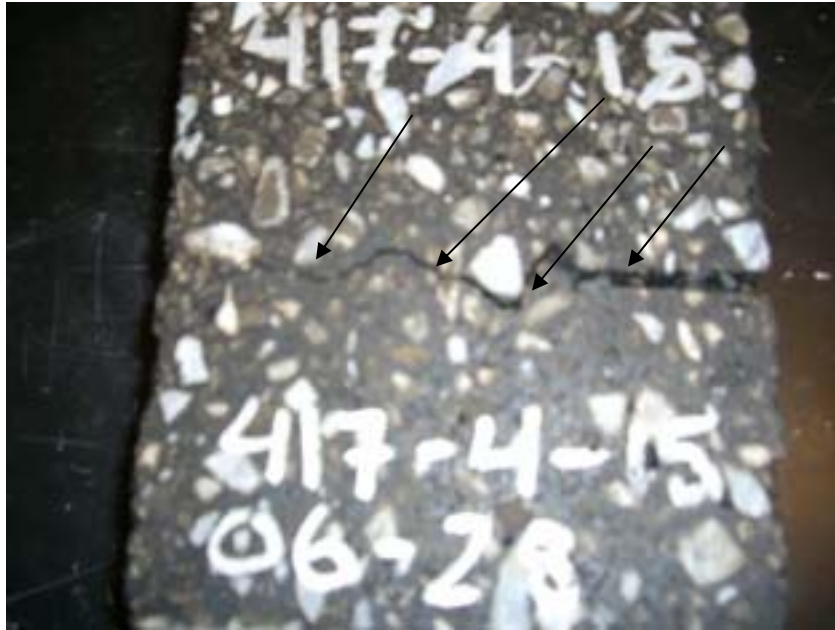
Figure 3.14 Gradual crack propagation after the SENT test.
