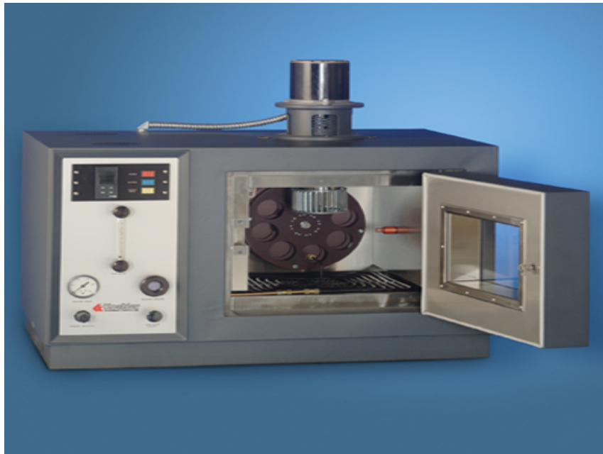
Figure 3.1 Typical rolling thin film oven (RTFO) used for short-time aging of asphalt binders. 69
