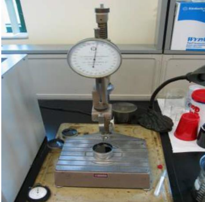
Figure 2.8: Penetration test equipment [62].
