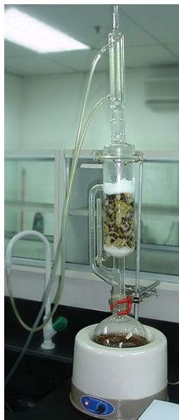
Figure 2.1 Soxhlet extractor for the extraction of lipids using organic solvent.
