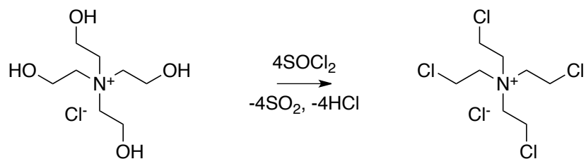
Scheme 2.29. Chlorination of tetraethanolammonium chloride ( 18 ) with thionyl chloride
