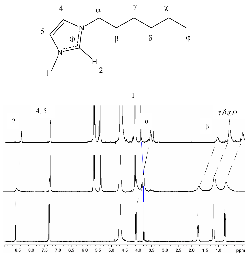
Figure 4.4 The ^1\text{H} NMR spectra of the free \text{IC6}^+ guest (lower spectrum) and after the addition of 0.3 equivalents of CB[7] (middle) and 1.1 equivalents of CB[7] (upper).
