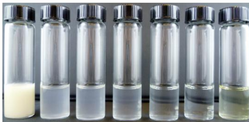
Fig. 5.4. Photographs of supernatants after 2 h of settling of 5 wt% kaolinite suspensions (sample 1). From left to right: no treatment, 0 mM, 0.01 mM, 0.1 mM, 1 mM, 10 mM, and 100 mM TMDAB. All suspensions containing TMDAB were subjected to CO 2 treatment.
