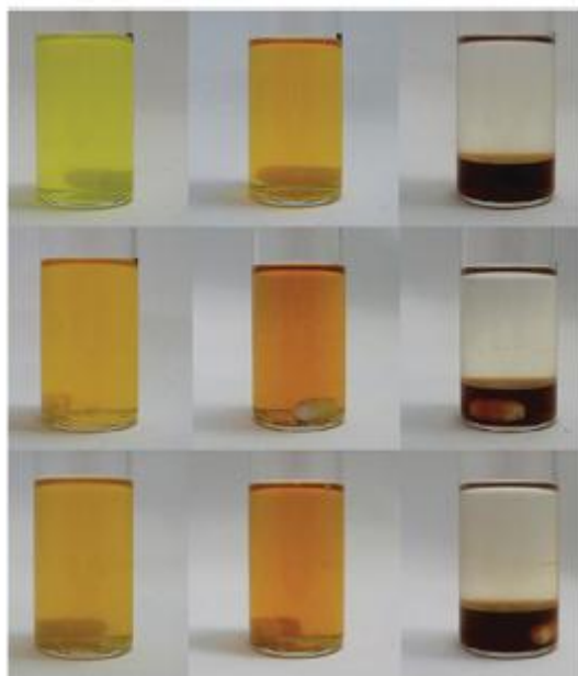
Fig. 4.7. Photographs of the hydroformylation of styrene in a mixture of tert -butanol and switchable water where compound 2.3 was the additive used. (Left) All reagents mixed before reaction or CO 2 treatment. (Centre) After completion of the hydroformylation reaction. (Right) After CO 2 treatment for 45 min. From Top to Bottom: Cycles 1 to 3 using the same catalyst and aqueous phase.
