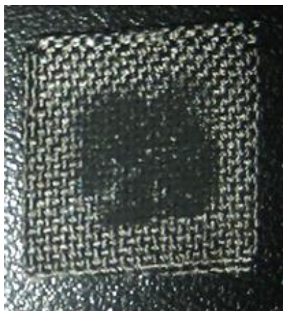
Figure 3.4: The PVP8/Nafion ® CCGDL after exposure to propiophenone for 24 h at 140 °C.
