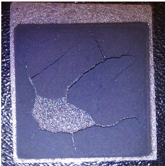
Figure 3.15: An image depicting the DPS PBI-based CCGDL from Figure 3.14A after it was exposed to a mixture of the working fluid (85 wt% 1-phenyl-1-propanol, 15 wt% propiophenone) at 140 °C for 20 h.
