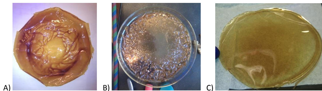
Figure 3.18: Different attempts at casting PBI S26 membranes. A) A membrane casted from a 5 wt% PBI S26 solution in DMAc at 80 °C. B) A membrane casted from a 5 wt% PBI S26 solution in HCO 2 H at room temperature. C) A membrane casted from a 5 wt% PBI S26 solution in DMAc at 50 °C with a steady Ar flow in an atmosphere bag.
