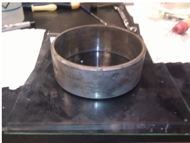
Figure A6: A template for casting PBI S26 that consisted of a plate glass floor and a steel cylinder wall. The template was used to make PBI S26 membranes (procedure described in chapter 2.4.2).
