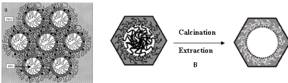
Figure 4-3: P123 core-mantle surfactant assembly (Diagram A , adapted from ref. 18). PEO-block occlusion into silica network illustrated. Micropores form after surfactant removal, either by calcination or by extraction (Diagram B , adapted from ref. 19).
