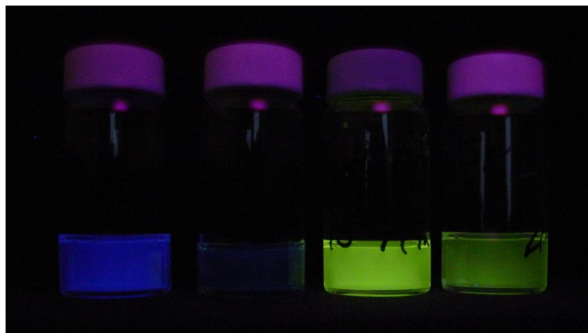
Figure 3.3a. Photograph, under 365 nm irradiation, of the compounds 1-MOM , 1-OH , 1-BPh 2 and 1-Alq 3 .
