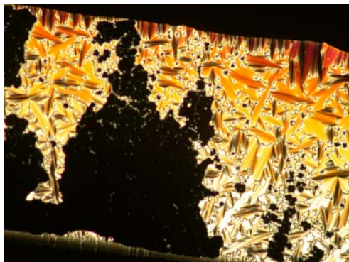
Figure 3-19. Textures of compound 40a observed by polarized microscopy on cooling: SmA phase at 85 °C. (100X Magnification)
