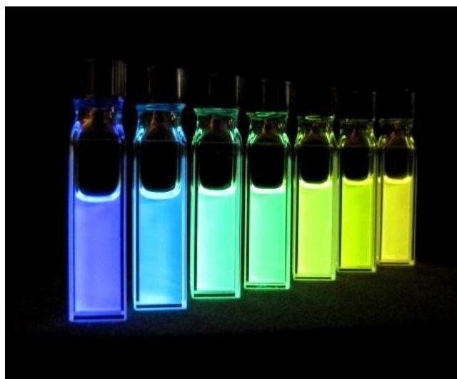
Figure 4.4: (Top): Normalized emission spectra for BNppy at 10^{-5} M in various solvents. Bottom: Solutions of BNppy at ca. 10^{-5} M under irradiation with UV light (365 nm). From left to right: hexanes, toluene, THF, CH 2 Cl 2 , acetone, MeOH, MeCN.
