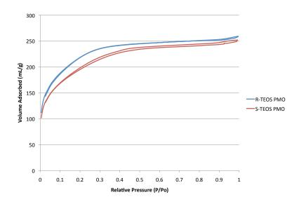
Figure 5.29: Nitrogen sorption isotherms for BINAPO/TEOS PMOs.
