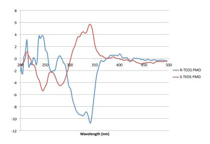
Figure 5.30: Circular dichroism spectrum of BINAPO/TEOS PMOs.
