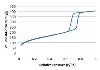
Figure 2.18: Nitrogen porosimitry of aminopropyl functionalized SBA-15 scavenger.
