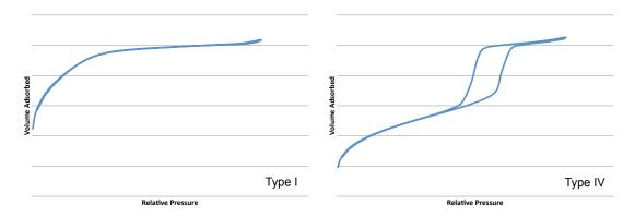
Figure 1.6: Examples of IUPAC type I and type IV isotherms.
