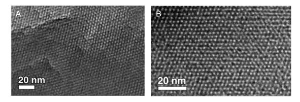
Figure 1.1: TEM images of MCM-41 (A) and MCM-48 (B). Reproduced from reference 27.
