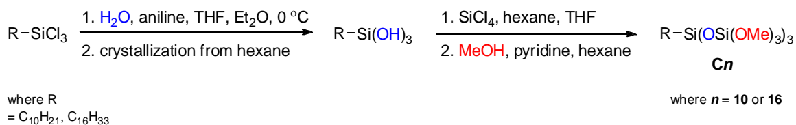
Scheme 3-3. Synthesis of Cn precursors from the corresponding alkyltrichlorosilane.
