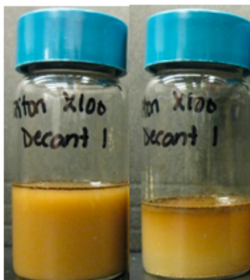
Figure 25: Photo of the wash mixture decant from a RT washing using Triton X-100 before and after salt addition. Even at saturation, the emulsion has not broken. Two distinct, continuous and immiscible phases are not observed.
