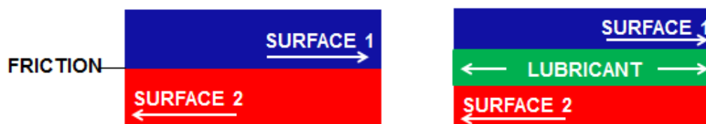
Figure 1.2. Basic schematic illustrating how lubricants act as mechanical barriers to lower friction and wear.
