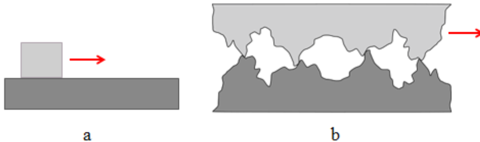
Figure 1.1. Two views of surfaces sliding past each other on (a) the macroscopic and (b) the microscopic level.
