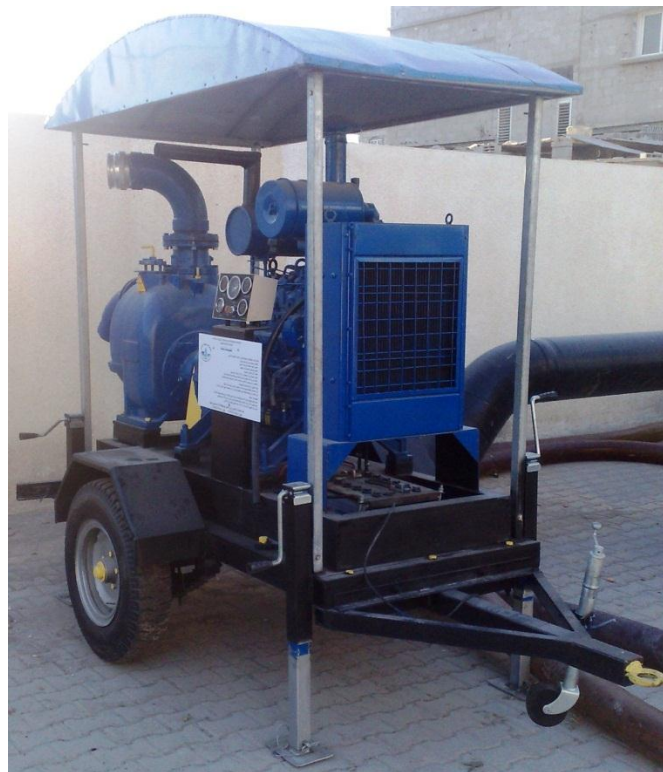
Figure (4.7): Mobile diesel pump
