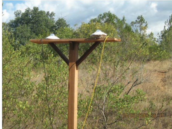
Figure 3.1: Configuration of albedometer in the field for calibration.
