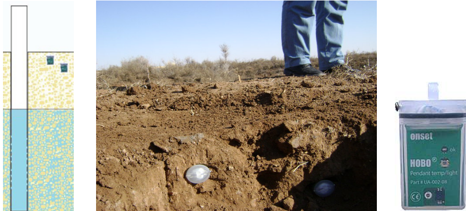
Figure 3.7: Two temperature loggers (HOBO Pendant) deployed in the soil at two different depths (approximately 5 and 10 cm).
