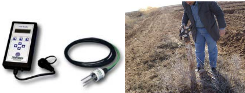
Figure 3.6: Left: Soil moisture measurements device (Stevens' Portable Hydra Reader and Stevens' Hydra probe). Right: water table depth reading device.
