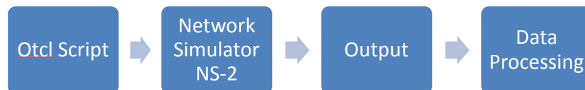
Figure 5.1: Description of simulation approach using NS-2 tool.
