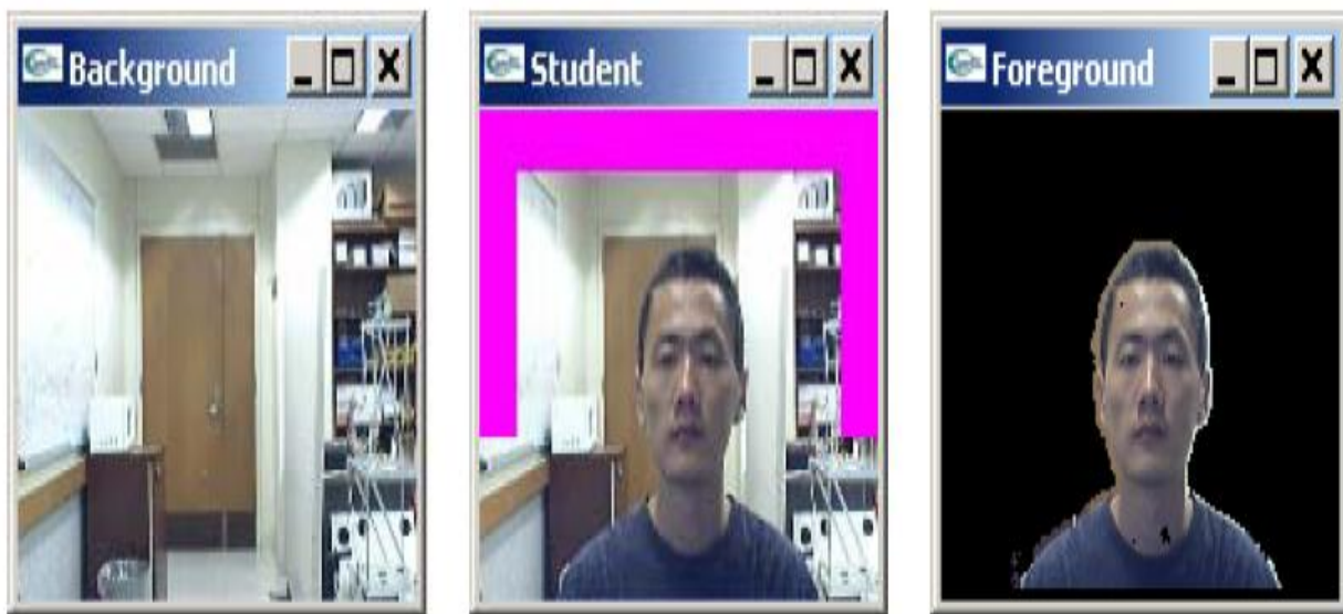
Figure 2.18: Frame, background, and video sprite compute by background subtraction.
