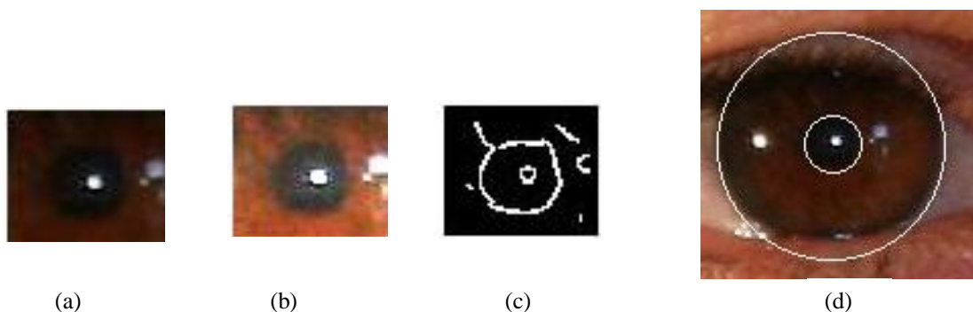
Figure 4.13: Steps of Pupil removal algorithm (a) the inner square of the iris. (b) result of adjust image in (a). (c) result of Canny edge detection. (d) result of the circular Hough transform.
