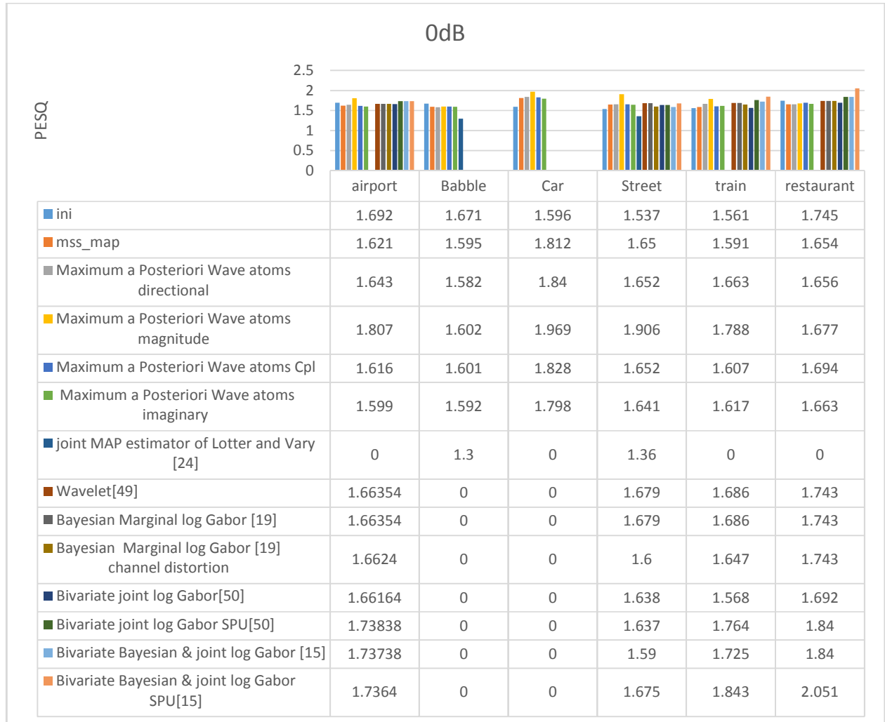
Figure 5.19 comparison of different algorithm corrupted with 0dB Noise and different noise type
