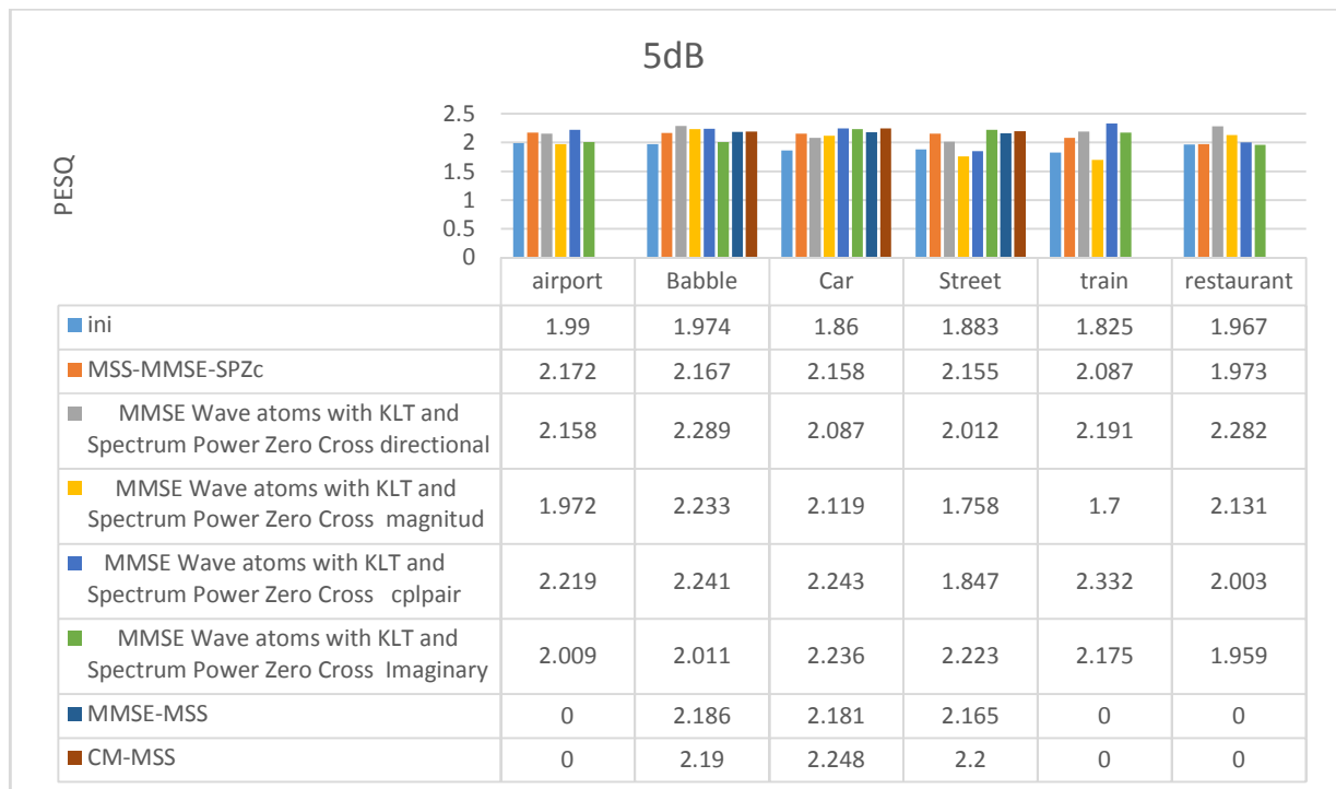
Figure 5.28 comparison of different algorithm corrupted with 5dB Noise and different noise type
