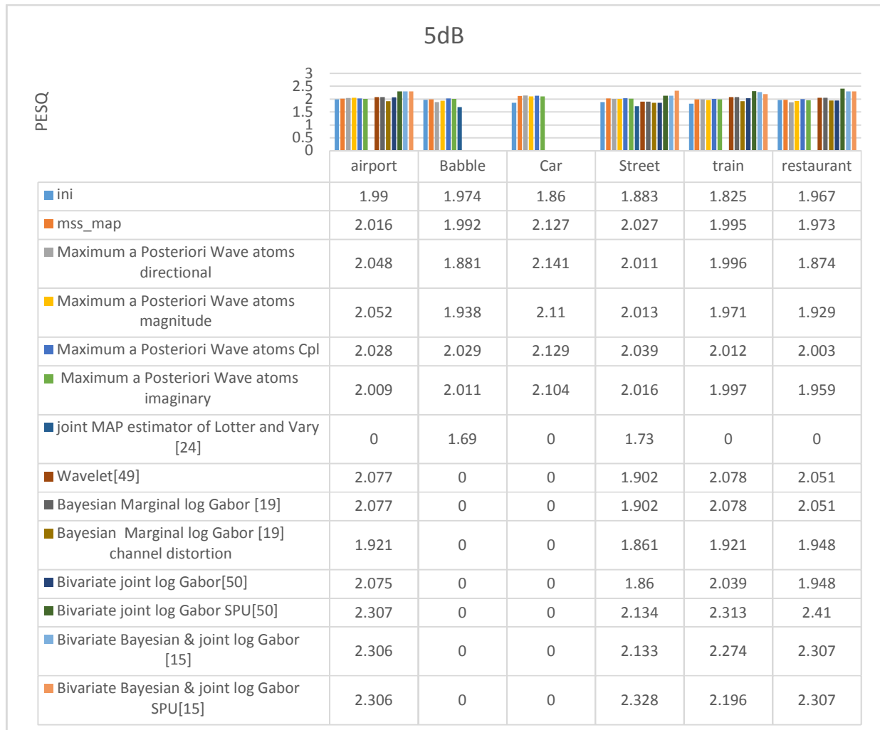
Figure 5.20 comparison of different algorithm corrupted with 5dB Noise and different noise type
