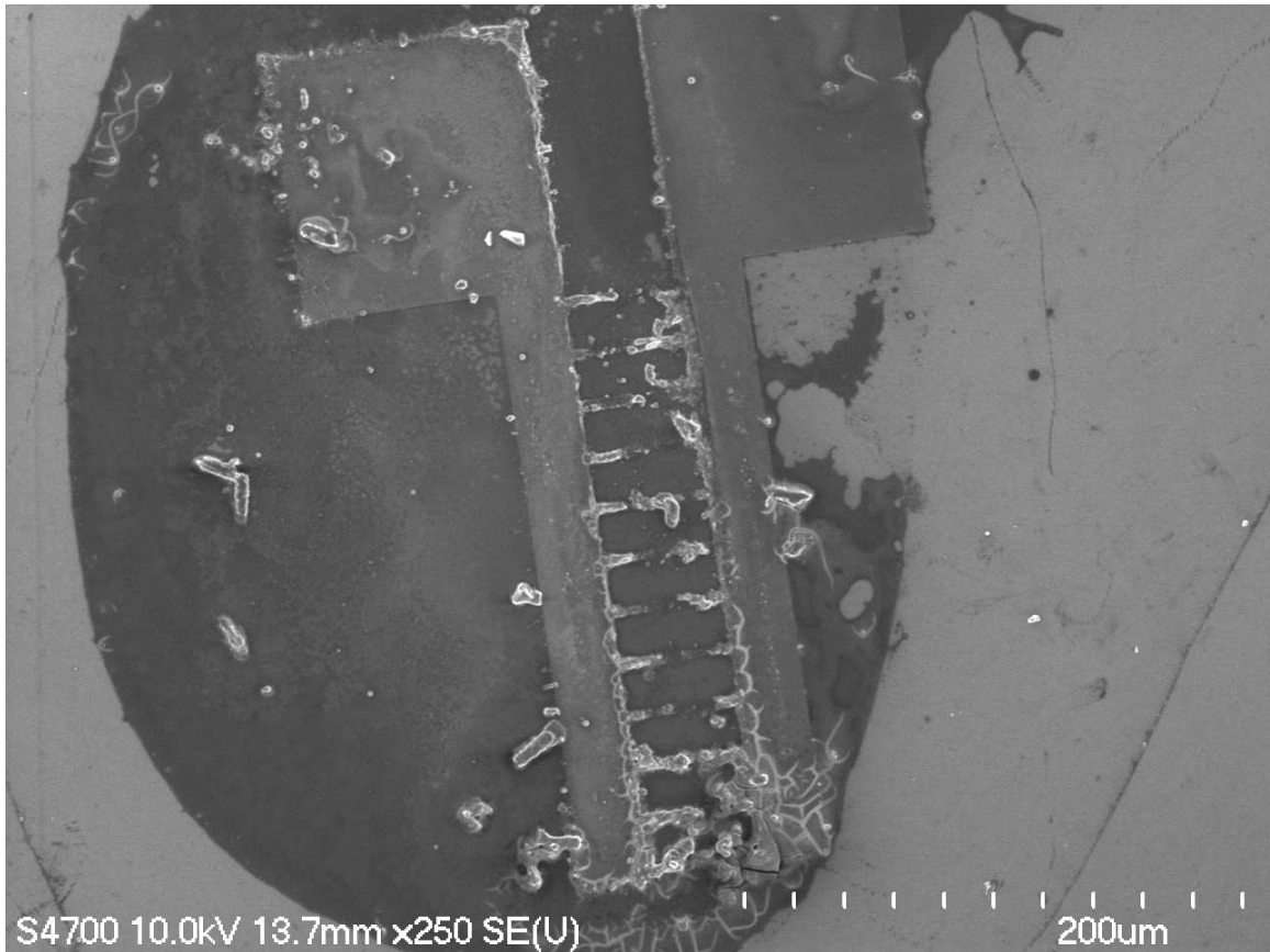
Figure 4.10: Dielectrophoresis in water requires much longer current flow times, and the resistive heating damages and destroys the electrodes.
