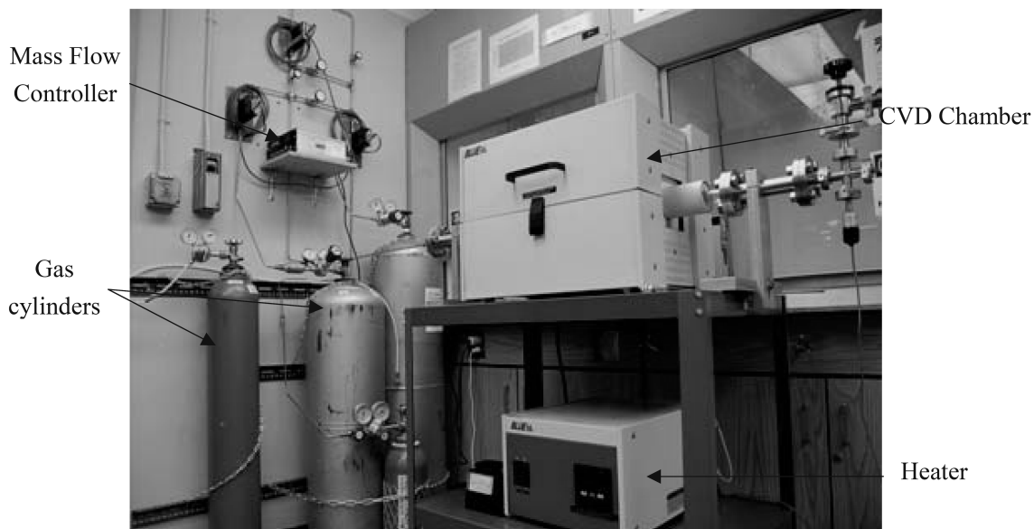
Figure 3.4: The thermal CVD system. Image reprinted with permission from reference [48].
