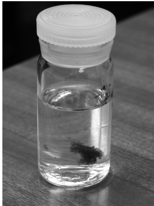
Figure 4.9: Carbon nanotubes in dispersion begin condensing immediately after condensation, and the aggregate becomes visible within 15-20 minutes.
