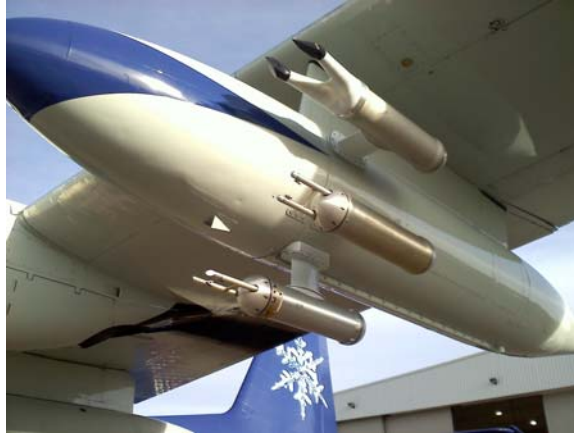
Figure 5.3: Instrument installation for IDEAS 2011. Top right: Holodec II. Middle: Standard 2DC. Bottom: Modified 2DC. The Holodec is mounted with the camera arm ( z = 0\text{mm} ) inboard.
