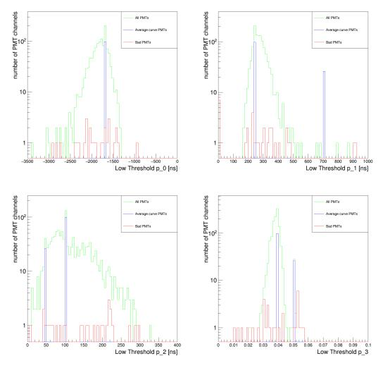
**Figure 3.5:** The distribution of the slewing fit parameters,  $p_0$  (upper left),  $p_1$  (upper right),  $p_2$  (lower left),  $p_3$  (lower right) for the low threshold fit. The green distribution contains all 1200 PMT IDs. The blue distribution contains all PMTs assigned the average curve, due to not being active at the time of calibration or not receiving laser light. The red distribution represents the channels known to be bad.
