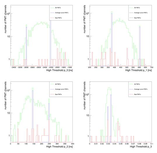
**Figure 3.6:** The distribution of the slewing fit parameters,  $p_0$  (upper left),  $p_1$  (upper right),  $p_2$  (lower left),  $p_3$  (lower right) for the high threshold fit. The green distribution contains all 1200 PMT IDs. The blue distribution contains all PMTs assigned the average curve, due to not being active at the time of calibration or not receiving laser light. The red distribution represents the channels known to be bad.
