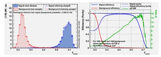
**Figure A.8:** Response values for the BDTs for signal and background testing and training data (left) and efficiency of the background and signal data vs response value (right) using  $f_{hit}$  bin 8.
