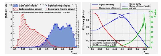
**Figure A.2:** Response values for the BDTs for signal and background testing and training data (left) and efficiency of the background and signal data vs response value (right) using  $f_{hit}$  bin 2.
