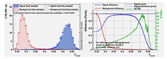
**Figure A.7:** Response values for the BDTs for signal and background testing and training data (left) and efficiency of the background and signal data vs response value (right) using  $f_{hit}$  bin 7.
