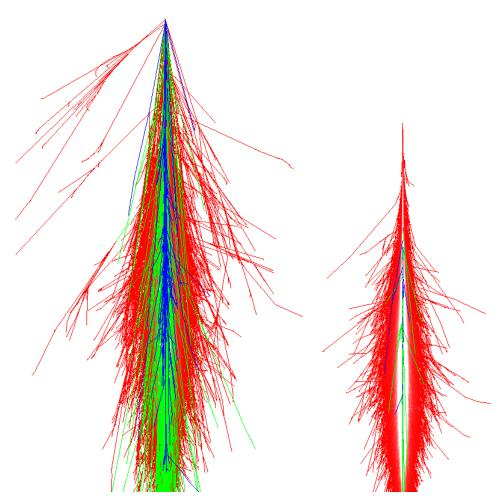
**Figure 1.4:** Simulations of 10 TeV proton (right) and photon (left) induced showers. Red is the electromagnetic portion (electrons, positrons, photons), blue is the hadronic component, and green is the muon component. COR-SIKA software was used to make these plots [7] [3]
