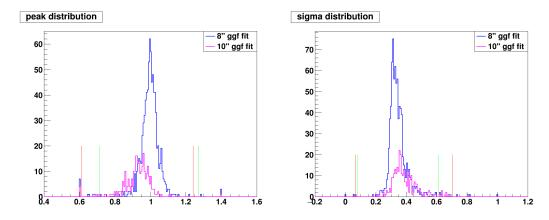
**Figure 3.3:** Distributions of the SPE value (left) and the width of the SPE gaussian (right) for 8" (blue) and 10" (magenta) PMTs. The cut value lines for the 8" PMTs (red) and 10" PMTs (green) are also shown [21].
