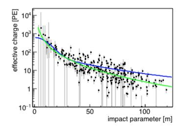
Figure 2.4: Charge distribution as a function of the distance of the PMT location (location of the charge measurement) from the core. Showing best fit of gaussian-NKG function after the  $\chi^2$  minimization (Blue) and the NKG fit using the core position from the gaussian-NKG function (Green) needed for determining the shower age and amplitude parameters [3].
