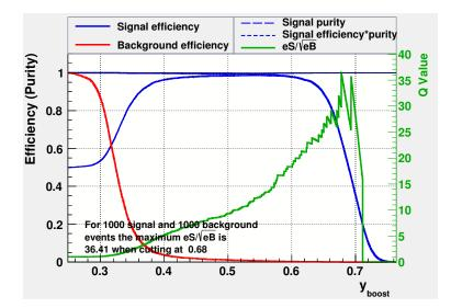
**Figure 4.2:** Efficiency plot for both the signal and background data vs the response value,  $y_{boost}$ , for  $f_{hit}$  bin 9.
