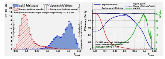
**Figure A.5:** Response values for the BDTs for signal and background testing and training data (left) and efficiency of the background and signal data vs response value (right) using  $f_{hit}$  bin 5.
