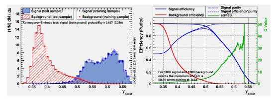
**Figure A.4:** Response values for the BDTs for signal and background testing and training data (left) and efficiency of the background and signal data vs response value (right) using  $f_{hit}$  bin 4.
