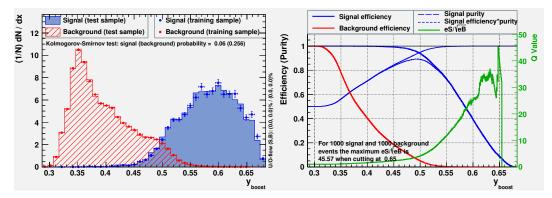
**Figure A.3:** Response values for the BDTs for signal and background testing and training data (left) and efficiency of the background and signal data vs response value (right) using  $f_{hit}$  bin 3.
