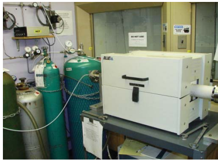
Figure 1.7: Picture of a horizontal CVD furnace used to grow carbon nanotubes
