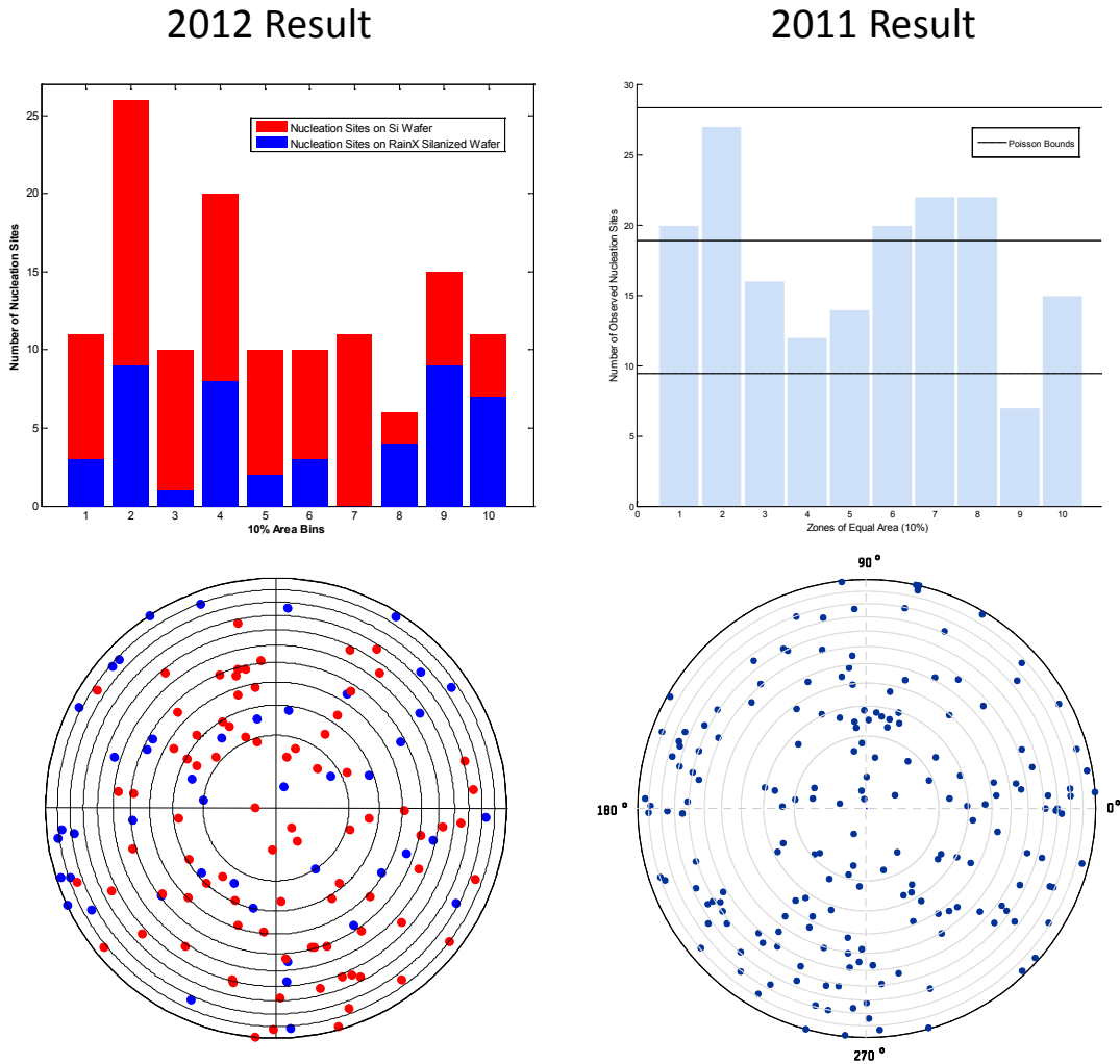
Figure 6.1: Droplet-Substrate Spatial Distribution Data Freezing sites are distributed uniformly over the droplet-substrate interface for data from Chapter 3 (right) and Chapter 4 (left). Here the data is derived from Figure 4.3 and Figure 3.4
