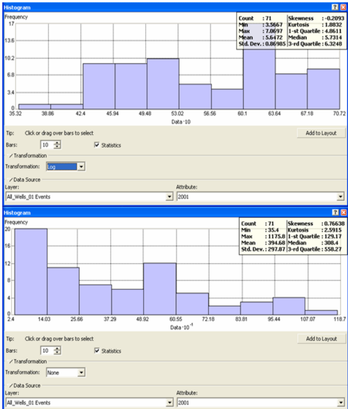
Histogram Graph for Chloride in year 2001 before and after log transformation and normalization process
