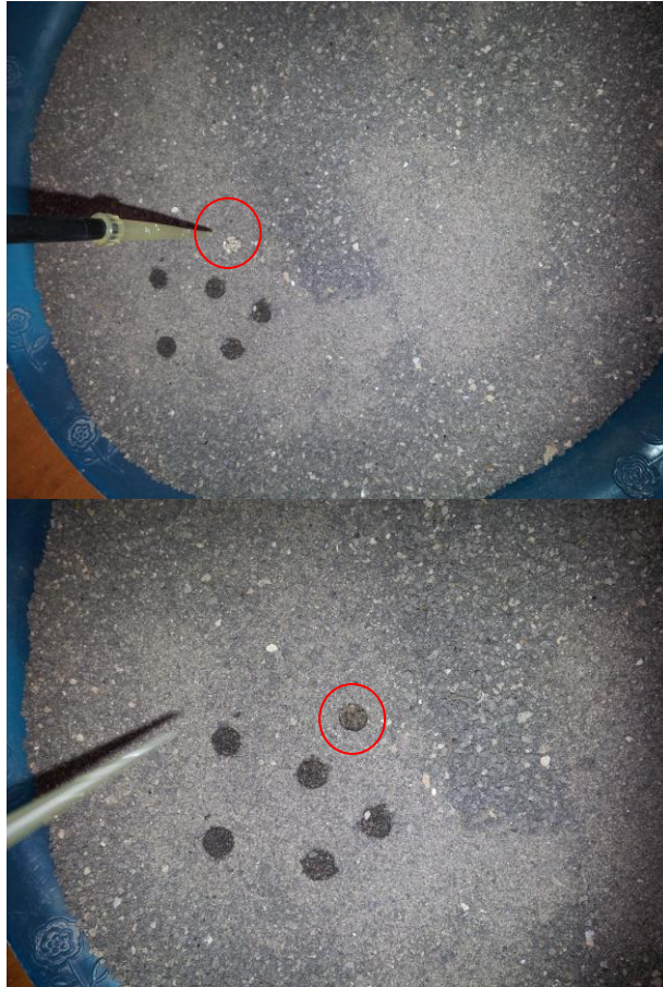
Figure 5.1 Water drop penetration, upper photo shows water drop at time zero, down photo shows penetrated drop.
