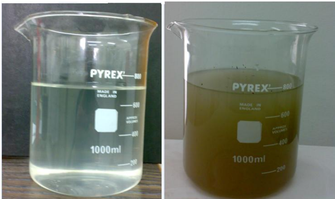
Figure (4.6) : Turbidity of storm water versus storm water after penetrating 2m of sand (photo)
