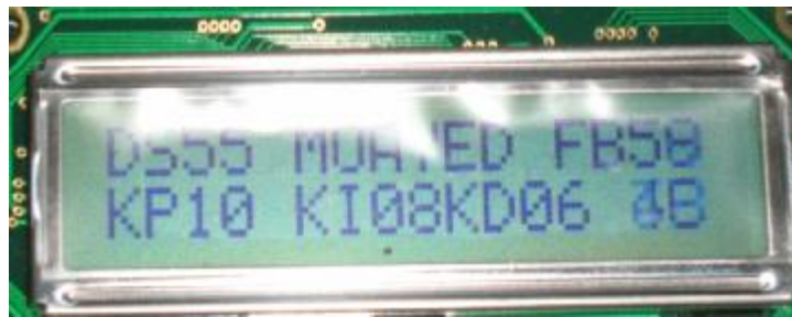
Figure 5.35: PID parameters on LCD of the FPGA card.
