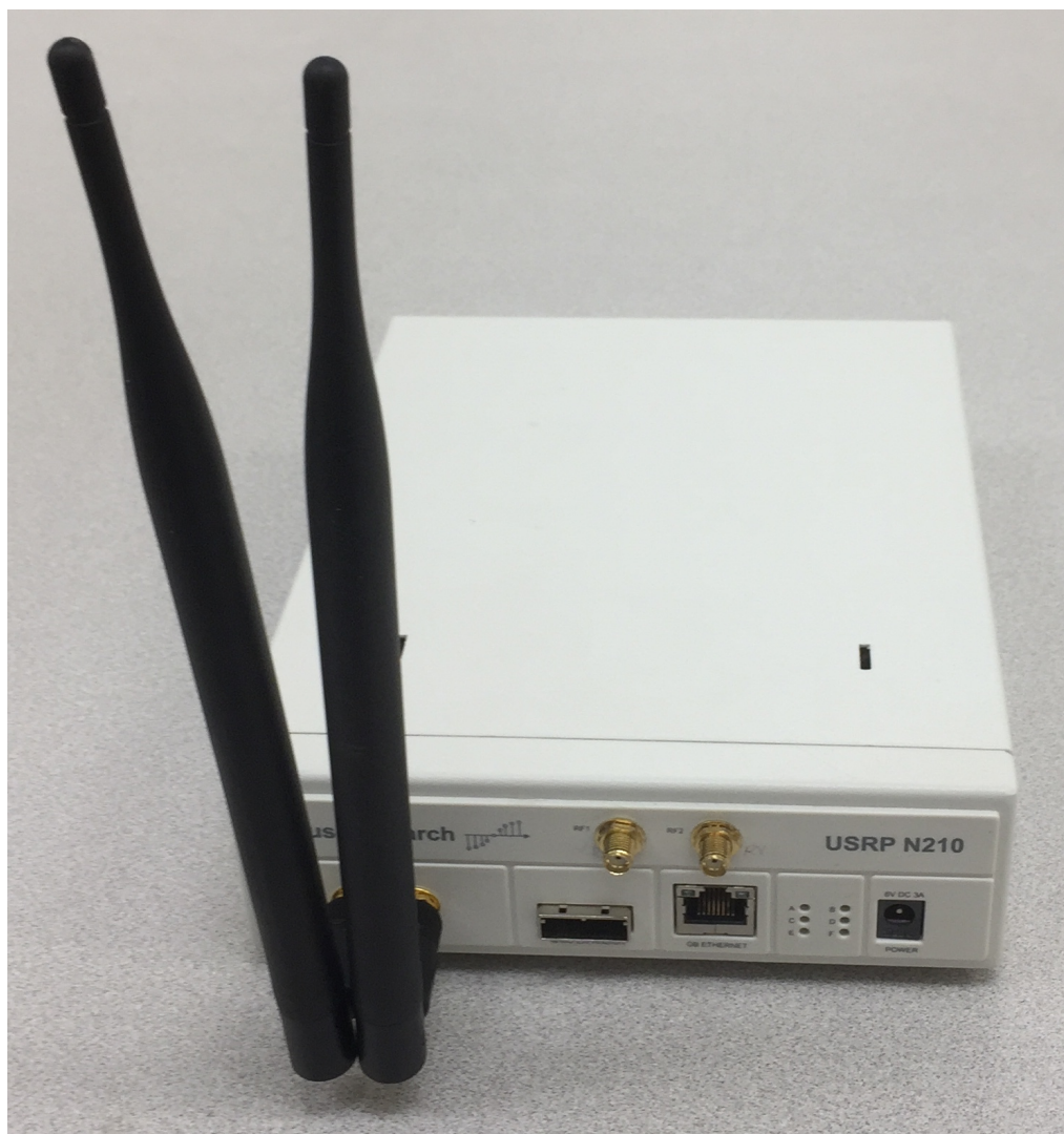
Figure 3.5: USRP N210 with two VERT900 atennas
