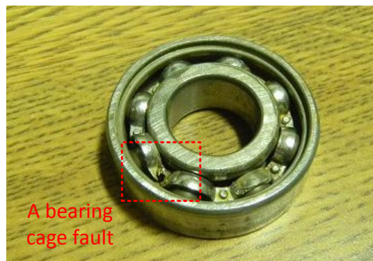
Figure 7.27: Testing bearing with a cage fault.
