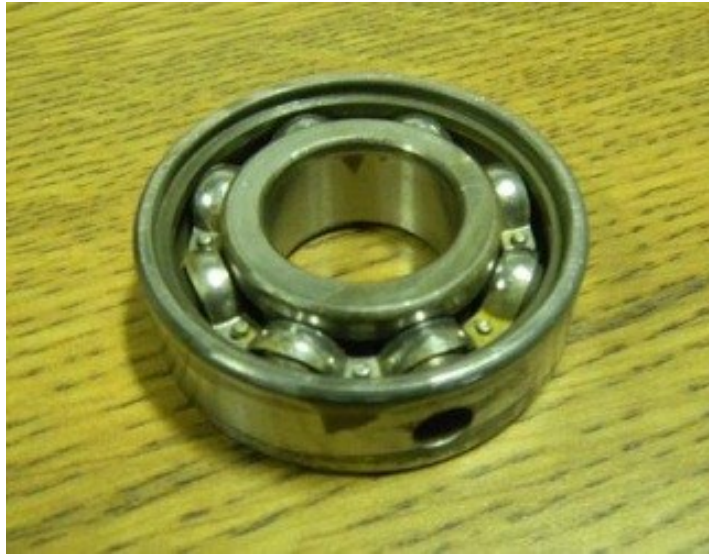
Figure 7.23: Testing bearing with an outer-race fault.
