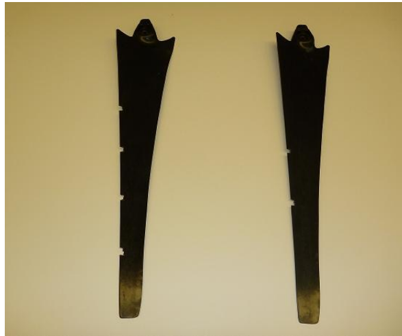
Figure 7.13: Two defected blades used for experiments.
