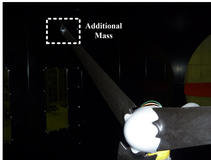
Figure 7.6: A blade with an additional mass to create a blade imbalance fault.
