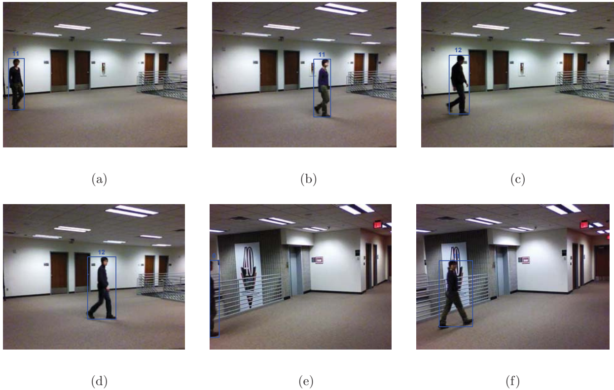
Figure 5.3: Two people tracked by the left camera and one tracked by the right camera (a-b),(c-d) People with labels 11 and 12 are tracked by the left camera; (e) a person enters the right camera view and is assigned a temporary label 0; (f) new person is assigned the correct label 11.
