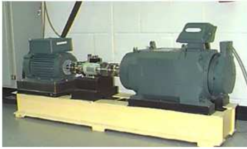
Figure 3.6: The test stand (the motor(left), the torque transducer/encoder (center), and the dynamometer (right))
