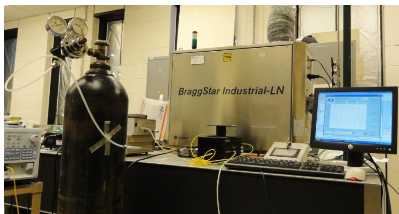
Figure 4.1 Measurement setup, includes air pressure source, Si125 interrogator, and computer
