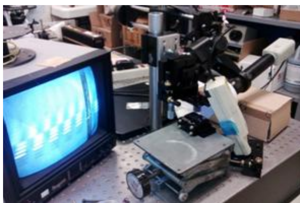
Figure 3.6 Setup for the adhesive process, includes microscope and monitor, translational stage, UV lamp
