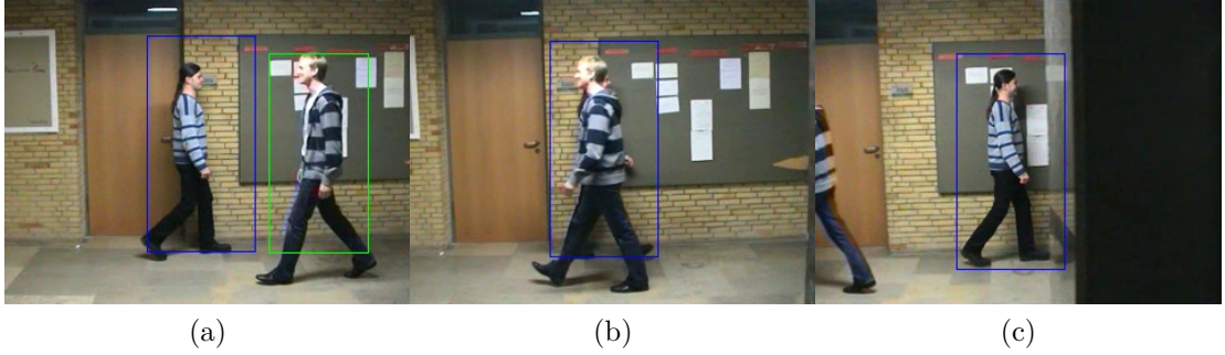
Figure 4.5: A scenario where similar objects coexist. The detector correction is turned on. A person wearing similar clothes appears in the middle of the video. Our framework is able to handle situations where similar objects coexist.
