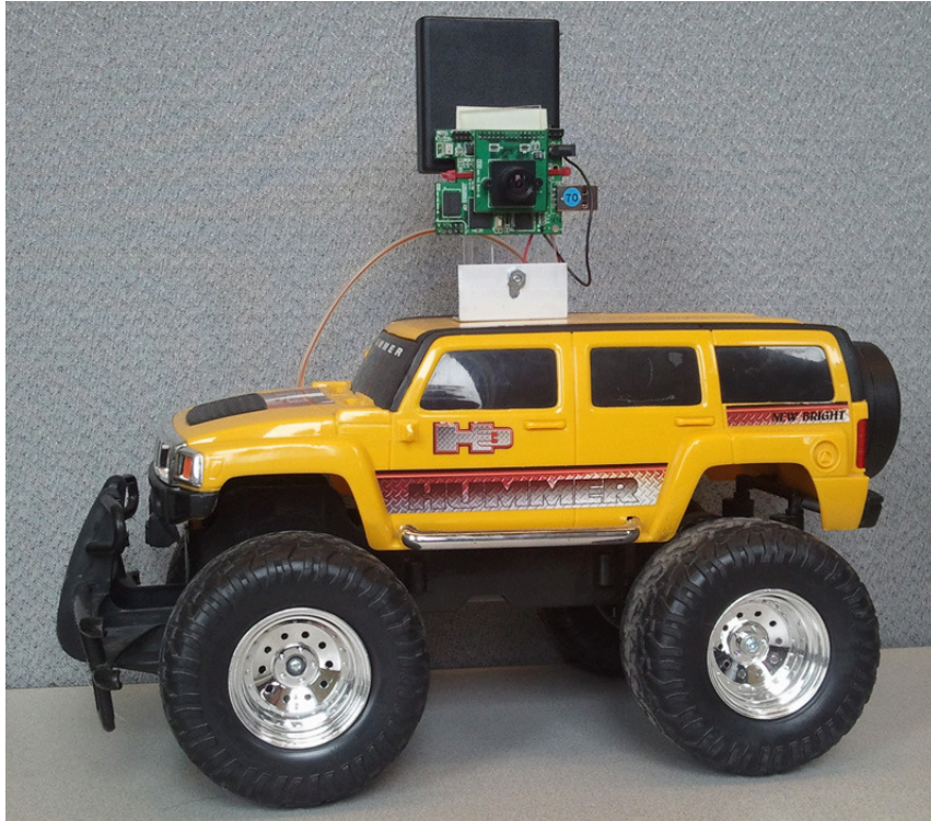
Figure 5.1: The CITRIC camera is mounted on a remote-controlled car.
