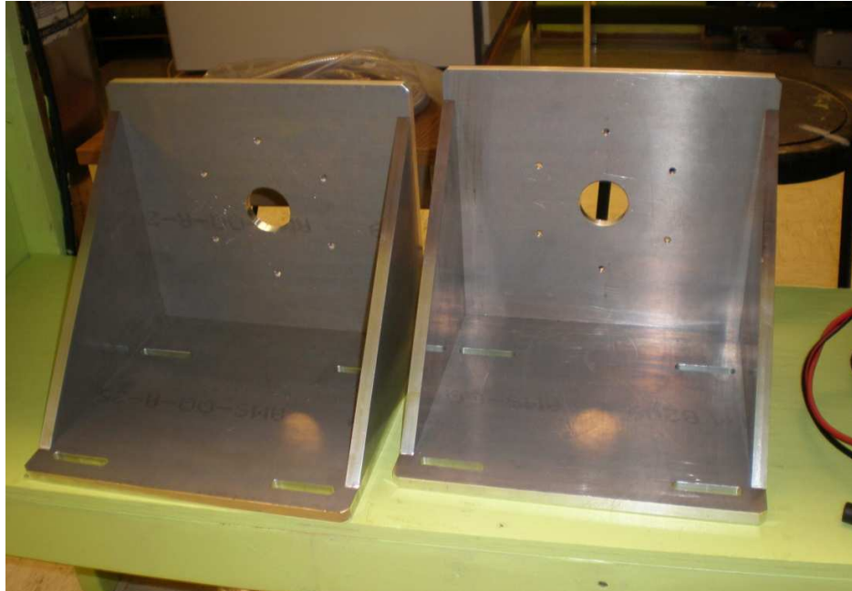
Fig. 5.1 Photographs of the machine assemblies to illustrate the fabrication process to-date. In (a) the rotor plates with shafts are shown along with the stator back-pieces with bearing insets, (b) shows the wound single- and double-layer stators and the motor mounting frames are shown in (c).
