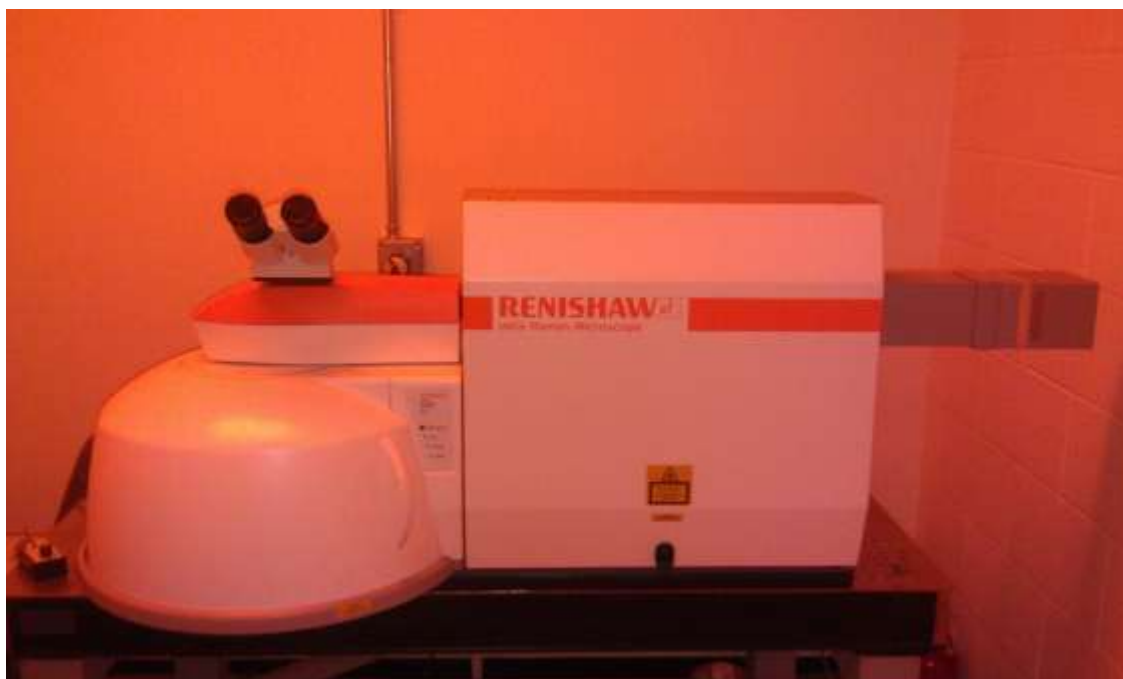
Figure 2.6. Renishaw inVia micro-Raman Spectroscopy.
