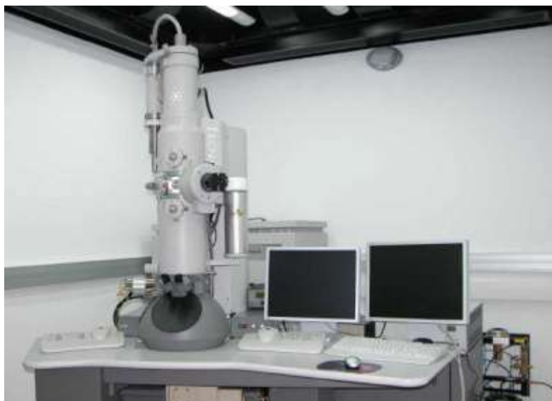
Figure 2.9. Tecnai G2 F30 TEM equipped with EDAX PV9900 spectrometer.
