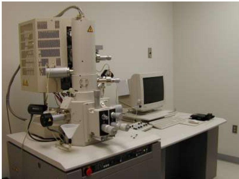
Figure 2.7. Hitachi FE4700 Field Emission Scanning Electron Microscope.
