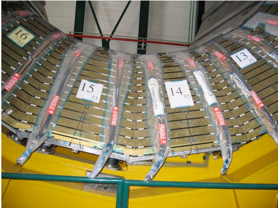
Figure 2.16: A closeup view of the wedges of the HCAL Barrel detector.
