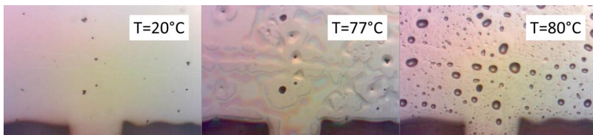
Figure 4.9: Still frames from digital video 4.1, a movie of a VDF oligomer thin film on a Pt/Co electrode being heated. For reference, the movie is taken at the location where the thin strip (bottom of the still frame) meets the square pad (see figure 4.1) of the bottom electrode. The film undergoes a dramatic change around 75 °C. At 80 °C, the pyroelectric signal disappears and bubble-like features appear on the surface of the film and remain even after the film is cooled back down to room temperature.
