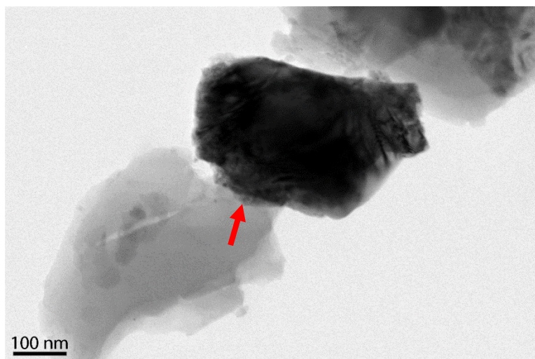
FIG. 5. 11 TEM image of the secondary phase in 500°C-annealed CoGeCrGe ribbons.
